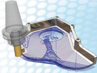
Non-concentric Milling Technology reduces cutting-tool load and evacuates chips more easily, dissipating heat more effectively. The increase in toolpath engagement occurs more gradually and
